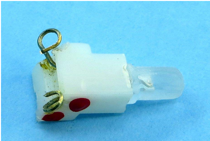
Photo 2: Lampholder removed from meter, T1 ¼ Led installed
