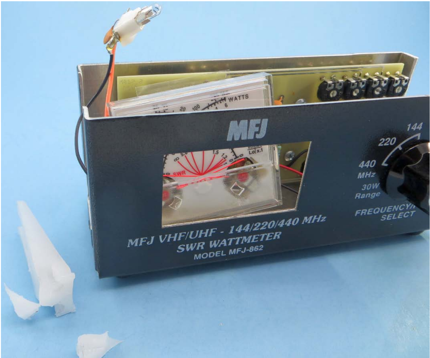
Photo 1: Loose meter with lampholder unplugged, broken support post
