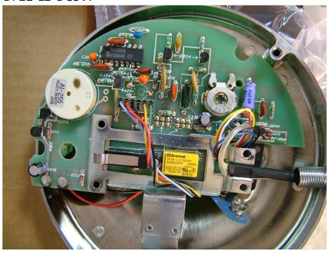
I tried tapping the relay with a screw-driver and got it to open the PTT line. Also, a small magnet held nearby can make it change state too. Still it would not work normally with either of the PTT switches.
