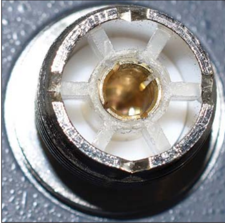
Figure 5: The end of a wattmeter connector with the previously solid plastic dielectric "honeycombed" in the area of the center conductor.
