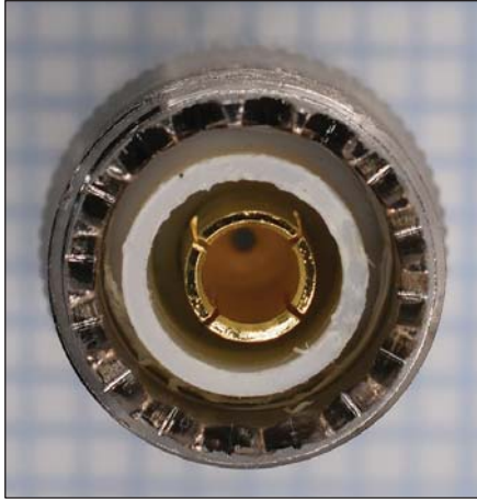
Figure 6: An SO-239 female to female connector with a "cored-out" dielectric.
